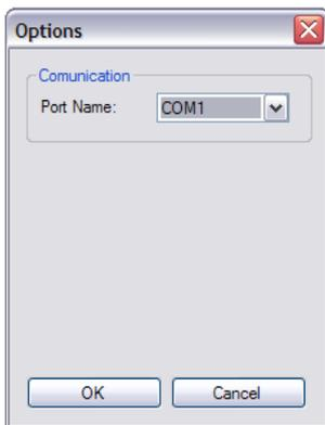
In *Options* window we can select on which serial port GSM module is connected.
