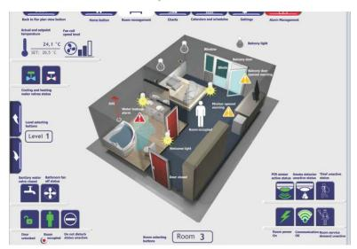
BMS acquire all this process data through standard Ethernet network using standard network protocols (Modbus TCP/IP).
