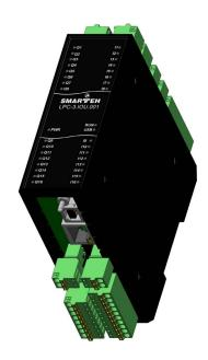
LPC-3.IOU is an innovative Universal PLC with software selection of the type and function for each of the 16 inputs and 2 analog outputs. Each of 16 inputs can be individually configured as digital (-12..30 V) input with a selectable range of switching voltages, as analog voltage (-10..10 V) or current (-20..20 mA) input.
