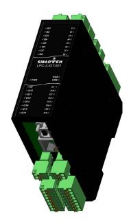
LPC-3.IOT is a Transistor PLC with 16 galvanic isolated digital inputs and 16 transistor outputs, with maximum output current of 1,2 A.
