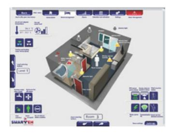
BMS acquire all this process data through standard Ethernet network using standard network protocols (Modbus TCP/IP).
