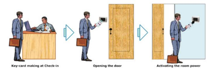
By standard RFID technology (Mifare, EM Marin), the same cards can be used for other purposes as entering the prepayment facilities (pools, spa, garage...) or for other identification purpose. Besides the access purpose for door locking, the RFID holders plays main role in hotel room occupancy detection that is related to energy saving feature in hotel room.
