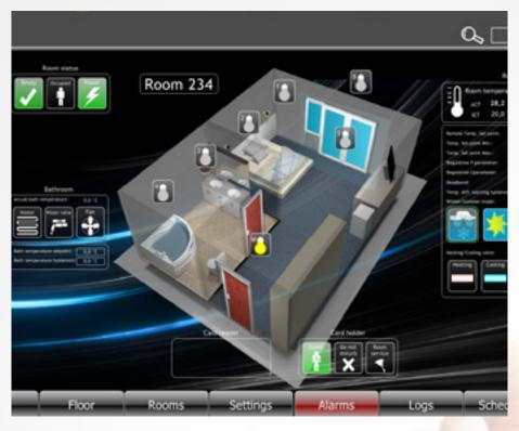
4) All automation systems are managed with a single Building Management System - BMS. With this centralized concept we achieve easy operation, energy saving, low-cost maintenance and fast reaction before a guest even notices an error.
