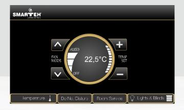
Graphical Operation Terminal supports Ethernet Modbus TCP/IP Master and/or Slave, Modbus RTU Master, CANopen Master and Slave. The application program can be transferred and debugging can be done remotely over the Ethernet. USB port can also be used for programming and debugging in the local.
