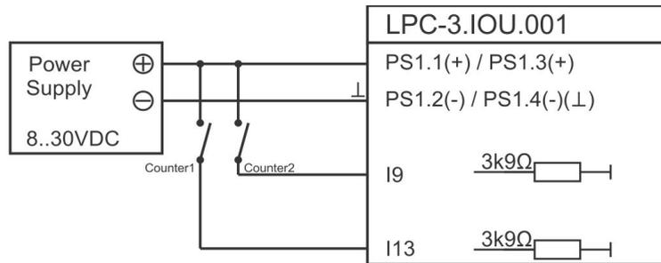
a) Voltage free contact fast counter connection to PLC input.
