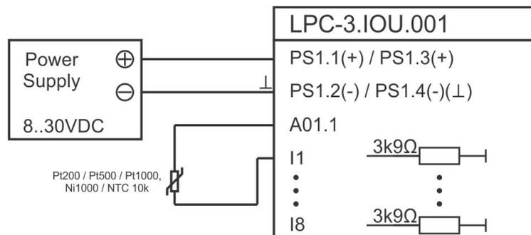
b) Pt200, Pt500, Pt1000, Ni1000, NTC10 kΩ connection of thermistor temperature sensing element to PLC input.
