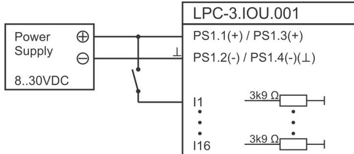
a) Voltage free contact connection to PLC input.
