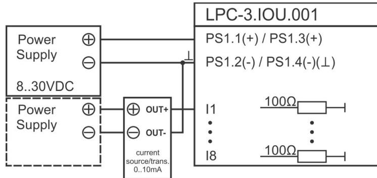
Unipolar connection of active current source/transducer 0 .. 10 mA to PLC input.
