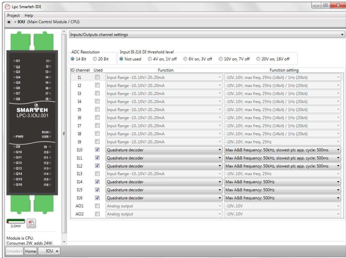
**NOTE:** This input detects a reference position for the Quadrature Decoder. When using reset input, if inputs A, B, and reset are all zero, the counter is also reset to zero. Reset can be triggered with hardware signal or from PLC application with QuadDec\_Reset.
