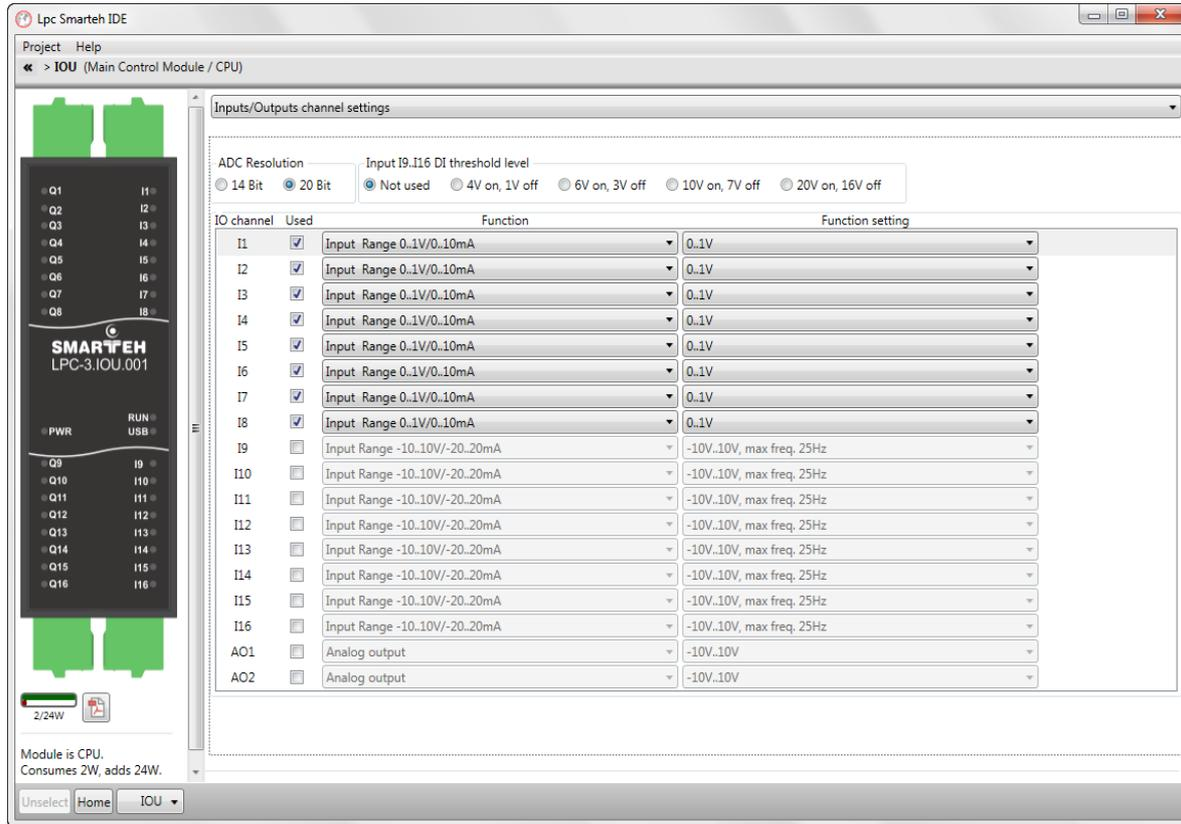
51 Configuration of the PLC is done using Smarteh IDE software tool. Please refer to PROGRAMMING GUIDE for details.
