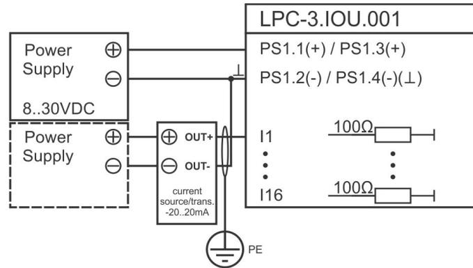
a) Unipolar connection of active current source/transducer -20 .. 20 mA to PLC input.
