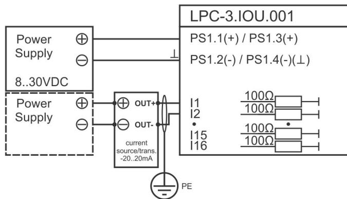
b) Differential connection of active voltage source/transducer -20 .. 20 mA to PLC input.
