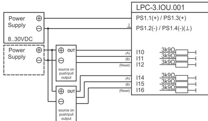
b) Active voltage source or push/pull fast counter output connection to PLC input.
