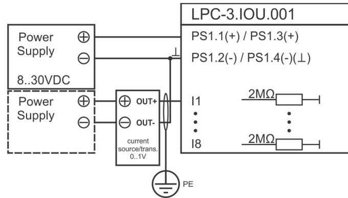
Unipolar connection of active voltage source/transducer 0 .. 1 V to PLC input.
