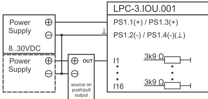
b) Active voltage source or push/pull output connection to PLC input.
