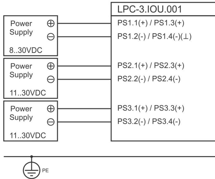
c) Not any PLC negative power supply poles connected together or to the Protective Earth (PE) ⊥ functional earthing.
