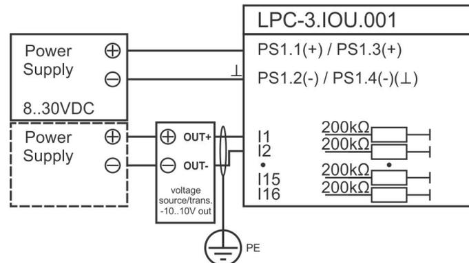
b) Differential connection of active voltage source/transducer -10 .. 10 V to PLC input.
