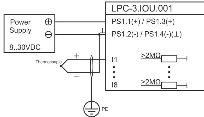
Unipolar connection of thermocouple temperature sensing element to PLC input.
