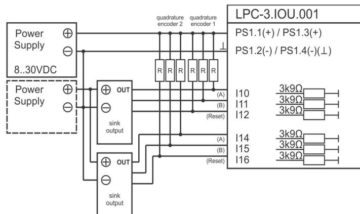
c) Active voltage sink fast counter output connection to PLC input.
