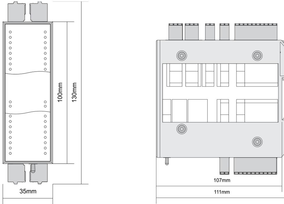
Module surrounding area must be free for optimal cooling.
