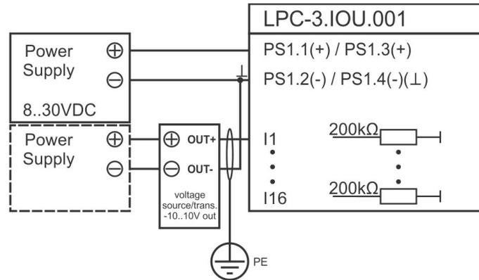
a) Unipolar connection of active voltage source/transducer -10 .. 10 V to PLC input.
