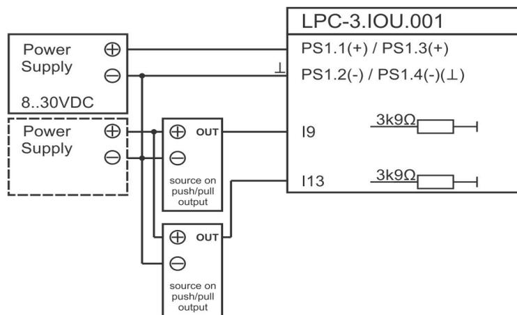
b) Active voltage source or push/pull fast counter output connection to PLC input.
