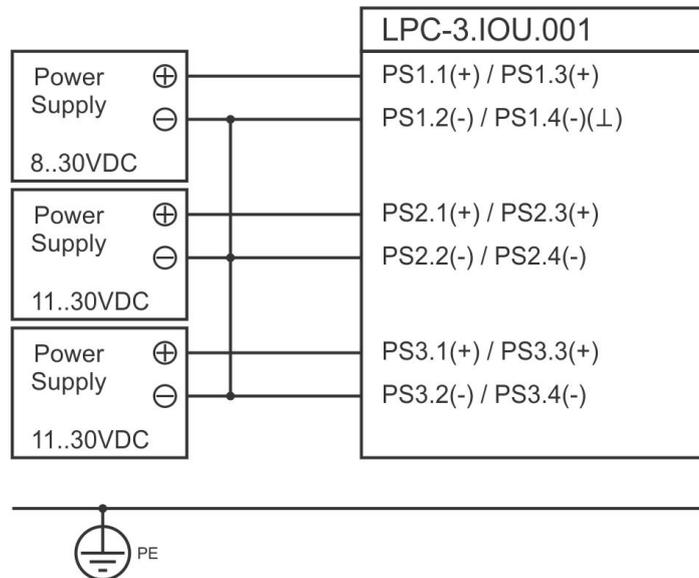
b) All PLC negative power supply poles connected together but not to the Protective Earth (PE) ⊥ functional earthing.
