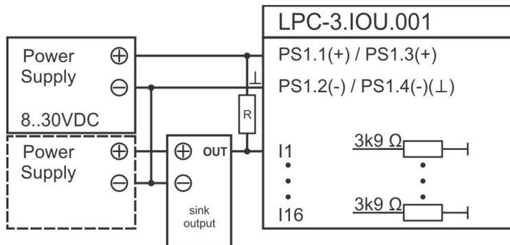
c) Active voltage sink output connection to PLC input.
