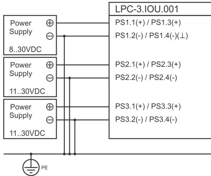
a) All PLC negative power supply poles connected together on to the Protective Earth (PE) ⊥ functional earthing.
