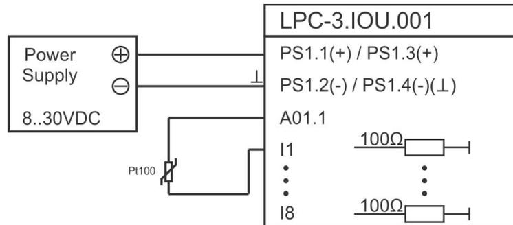
a) Pt100 connection of thermistor temperature sensing element to PLC input.
