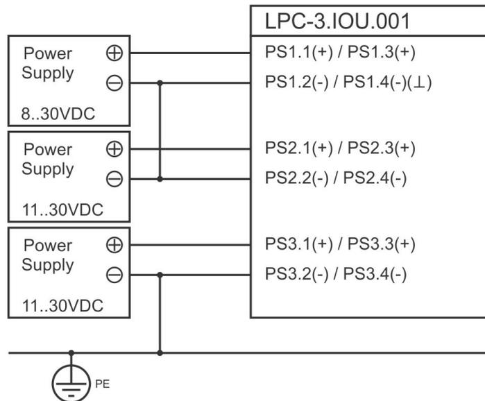
d) Mixed connection where required, selected PLC negative power supply poles connected together and/or to the Protective Earth (PE) ⊥ functional earthing.
