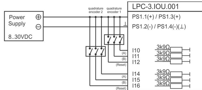
a) Voltage free contact fast counter connection to PLC input.
