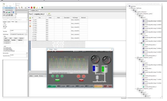
NOTE: Recommended minimum size of the touch object is 10 x 10 mm.
