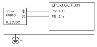
LPC-3.GOT negative power supply poles not connected to the Protective Earth (PE)  $\stackrel{\frown}{=}$  functional earthing.
