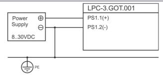
LPC-3.GOT negative power supply pole connected to the Protective Earth (PE) functional earthing.
