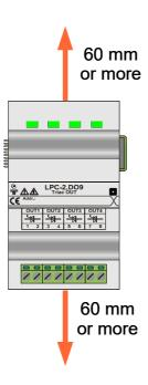
The clearances above must be considered before module mounting.
