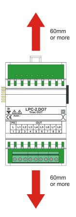
The clearances above must be considered before module mounting.
