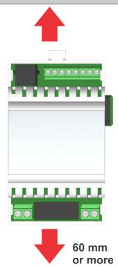
The clearances above must be considered before module mounting.
