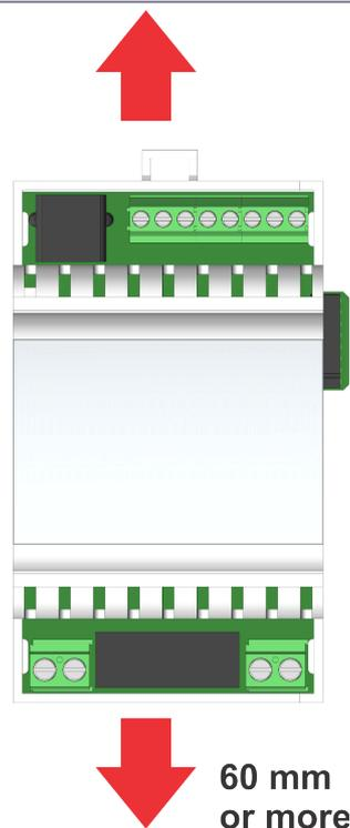
The clearances above must be considered before module mounting.
