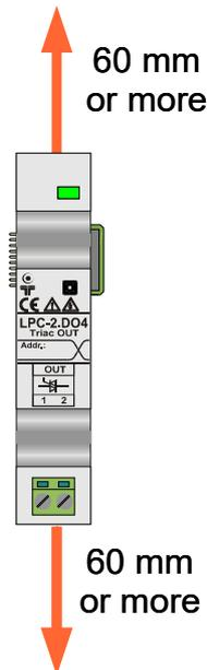
The clearances above must be considered before module mounting.
