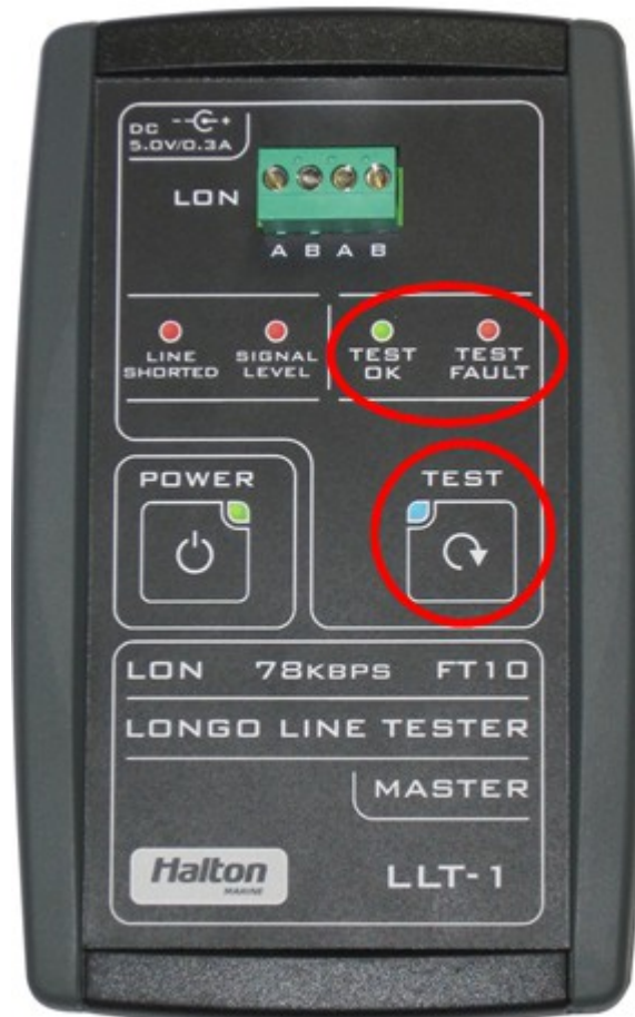
Picture 7: In continuous mode of testing press “TEST” button for approx. 3 sec. and LLT-1 tester will shows the result as “TEST OK” or “TEST FAULT”.
