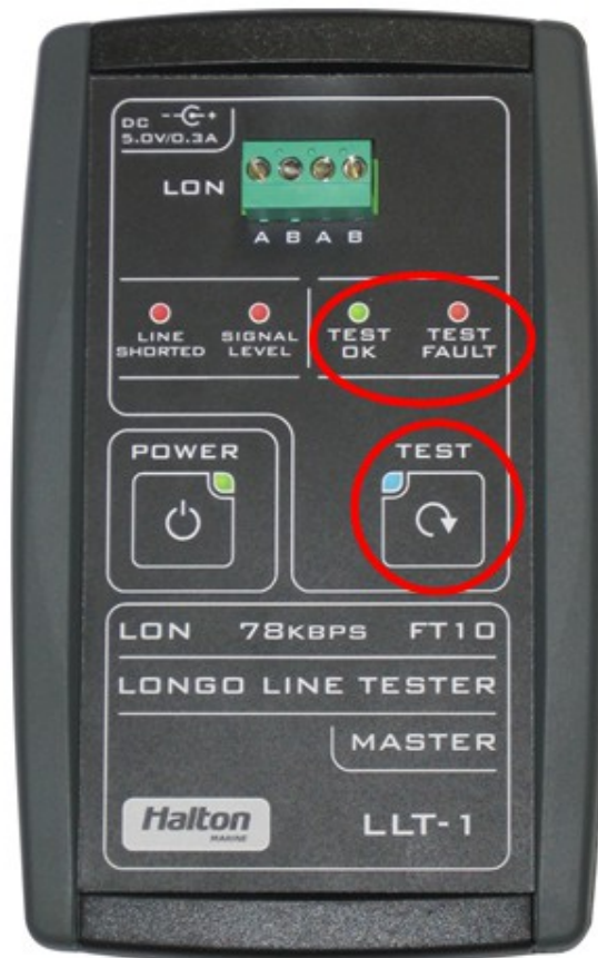
Picture 6: In single mode of testing press “TEST” button once and LLT-1 tester will shows the result as “TEST OK” or “TEST FAULT”.
